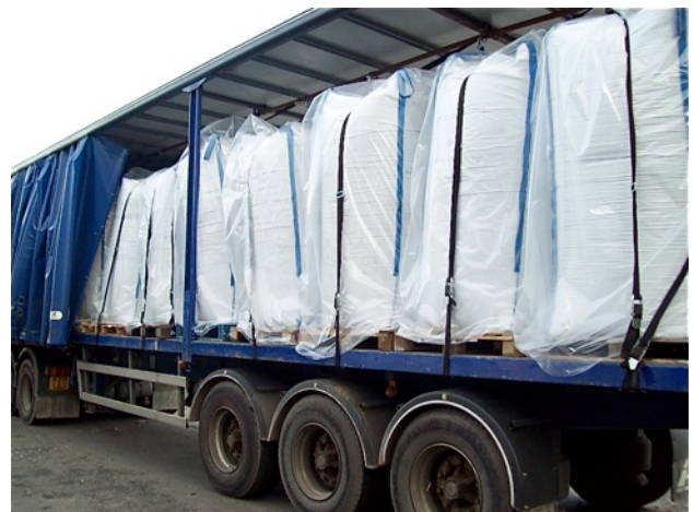
One tonne bags of Axpoly, inside heavy duty plastic bags and strapped to delivery vehicle.
